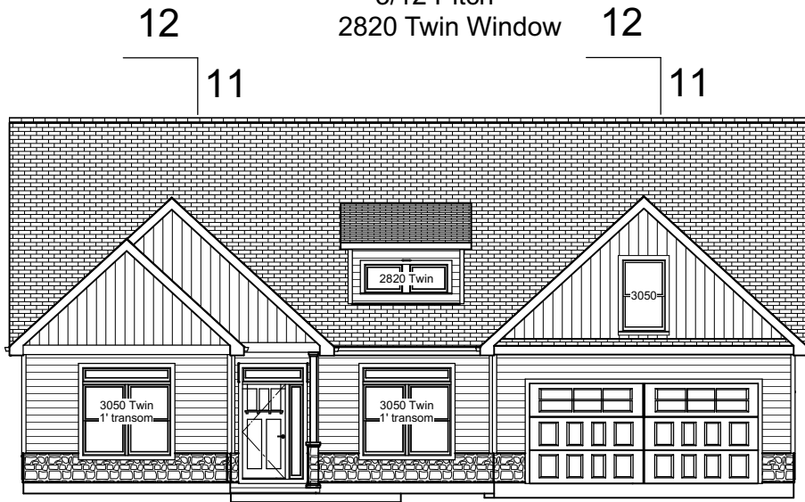
Exterior Elevation Front
